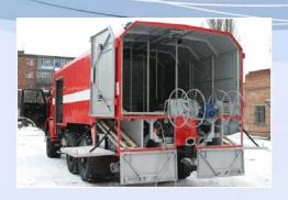
Arrange steam generator, cooling pool, suppression chamber make-up during long-term complete blackout
